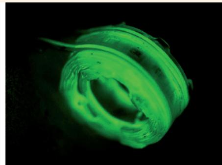
with the original solvent. The curving can be precisely controlled by the UV exposure, film morphology and heating conditions, which enabled the researchers to assemble various differently curving segments into complex three-dimensional architectures.
